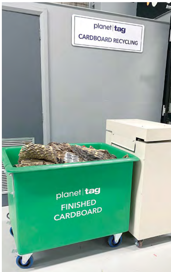
The Rongda cardboard recycler produces packaging material from shredded cardboard
