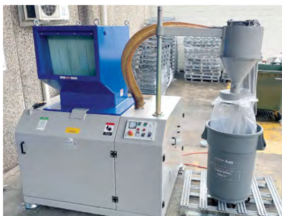
The Zerma GX300/600 granulates hard plastics, rubber, silicone and other waste material
